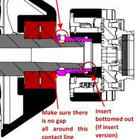
Tighten the EU chuck to the spindle on the lathe, make sure the rings on the spindle and chuck have been clamped. Note: EU Lock Ring is provided with the lathe
